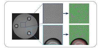
Figure 1: Whole-well images captured by Celigo from a Seahorse™ XF well with 3 posts. Accurate direct cell count is shown where cells are circled in green and exclusion of the post is shown in red.
