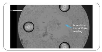
Figure 8: Celigo whole-well brightfield image shows non-uniformly seeded cells.
